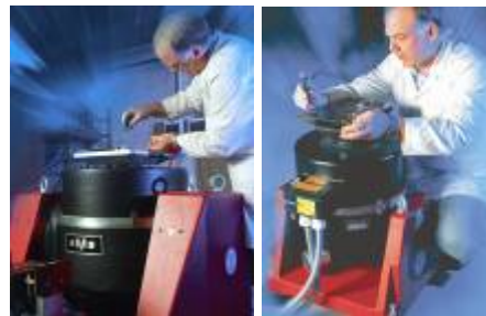
Installing of electronic devices for vibration test.
