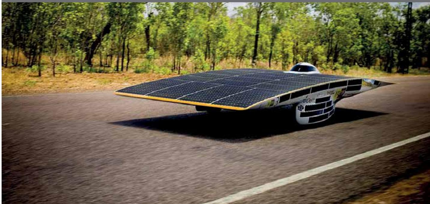
“Smartec temperature sensors are used in the solar race (Australia) to control the output of the photovoltaic cells.”
