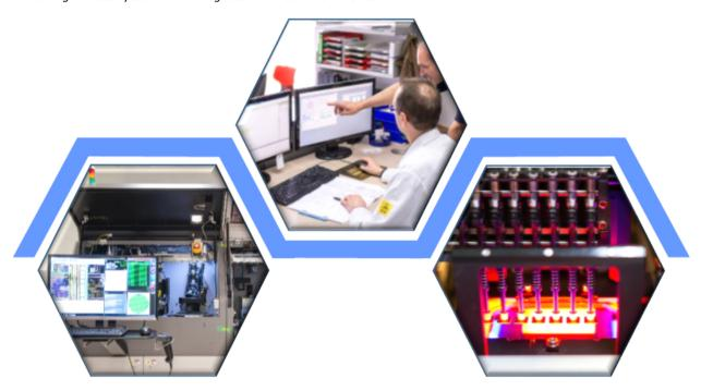
**Wafer & component testing** is the heart of the production function within RoodMicrotec, which means running an automated test floor 24 hour per day, 7 days per week. In this area, we perform the services of wafer testing, component testing, component programming, straightening, scanning and tape & reel of the semiconductor devices.
