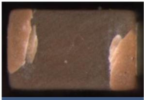
Cracks after removal of metallization
