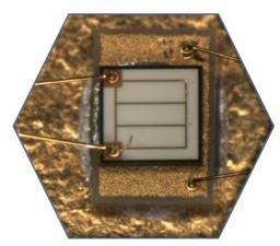
**Construction Analysis** and **Destructive Physical Analysis** (DPA) can be performed as part of a reliability assessment. The objective of construction analysis is early identification of potential deficiencies that can cause zero-hour failures or reliability problems. These tests are required for all components used in aerospace applications. Request numbers for DPAs are very stable as the aerospace market is less sensitive to economic cycles.
