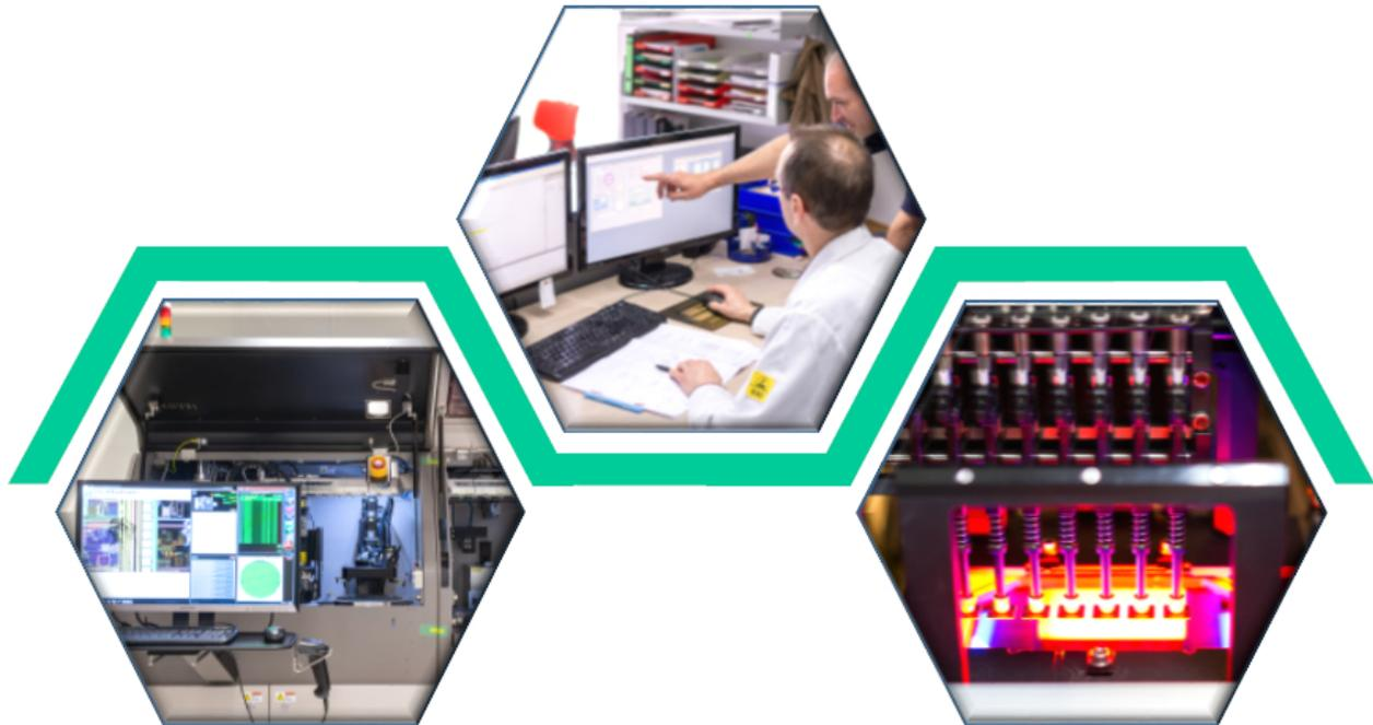
**Wafer & component testing** is the heart of the production function within RoodMicrotec, which means running an automated test floor 24 hour per day, 7 days per week. In this area, we perform the services of wafer testing, component testing, component programming, straightening & scanning and end of line of the semiconductor devices.
