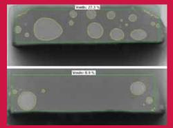
The figure shows on top one solder joint (field of view:  $1.6 \times 0.4 \text{ mm}$ ) of an SMD resistor where the X-ray inspection reveals 27% voids within the solder area underneath the part. The part at the bottom has only 9% voids. A shear test then showed that the shear force of the bottom part is 5% greater.
