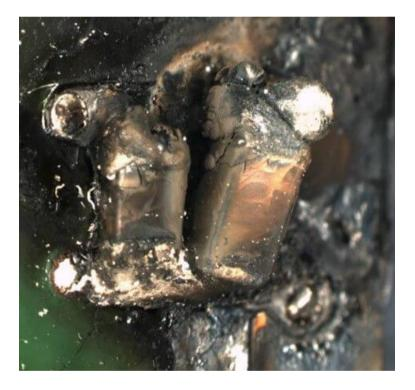
To minimize the risk of fires, various measures are required. These include the careful selection and quality testing of components, avoidance of excessive mechanical stress during the assembly, a proper heat dissipation, and the monitoring of operating conditions to prevent electrical overvoltages.
